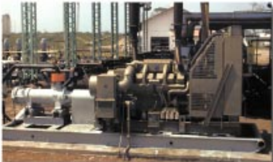
One of six 8L-462 on crude oil pipeline service in South America. Each delivers 575 GPM at 1850 PSIG.
